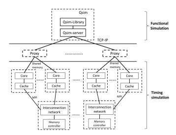
Figure 2: Manifold parallel simulation with Proxy.
