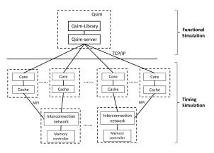
Figure 1: Manifold's timing-directed simulation model with client-server design.
